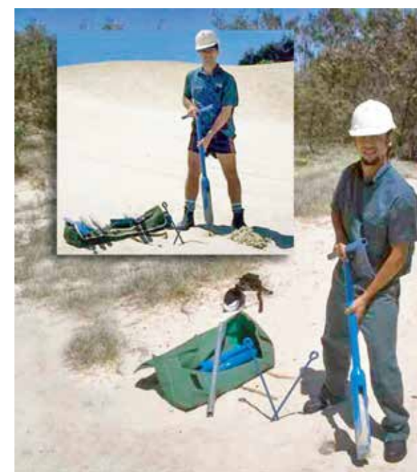
Sand auger sampling beach sand in 250-300mm increments. Also available in a heavy duty version made from thicker steel for debris or soil.
