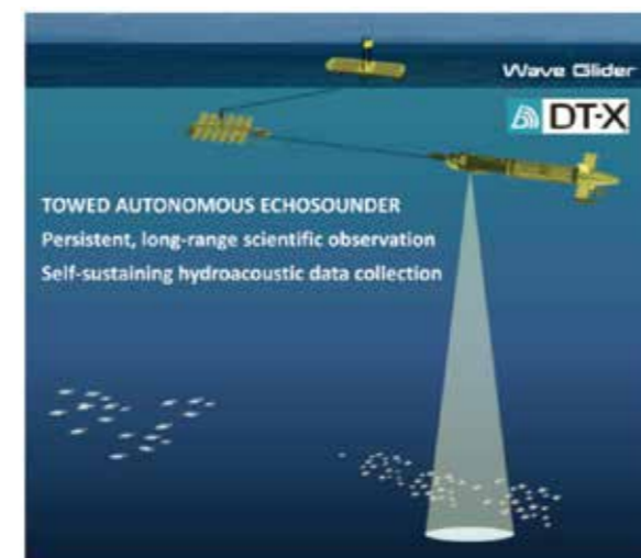
DT-X SUB搭载Wave Glider巡航
